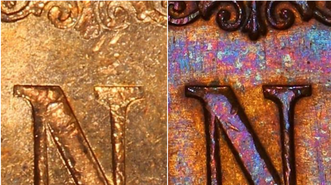
Figure 16. Evidence of the strength of the strike. Weakness at the top of the N on the 1916 business strike (left); no strike weakness on the specimen (right).
