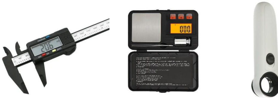
Figure 11. Tools of the trade. Digital vernier callipers, Digital jewellers Scales, Magnifier with built in light.
