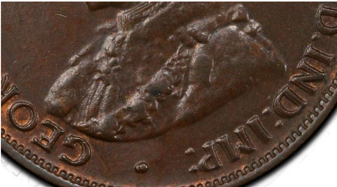
Figure 17. Doubled die obverse on a 1926 halfpenny. Photograph courtesy of PCGS.
