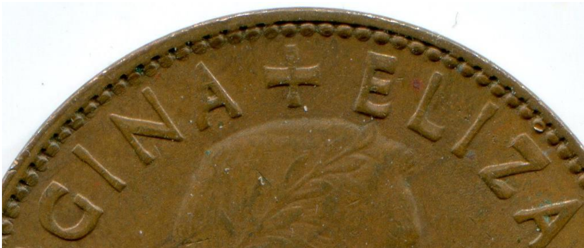
Figure 19. 1954 halfpenny with severe obverse mishubbing.
