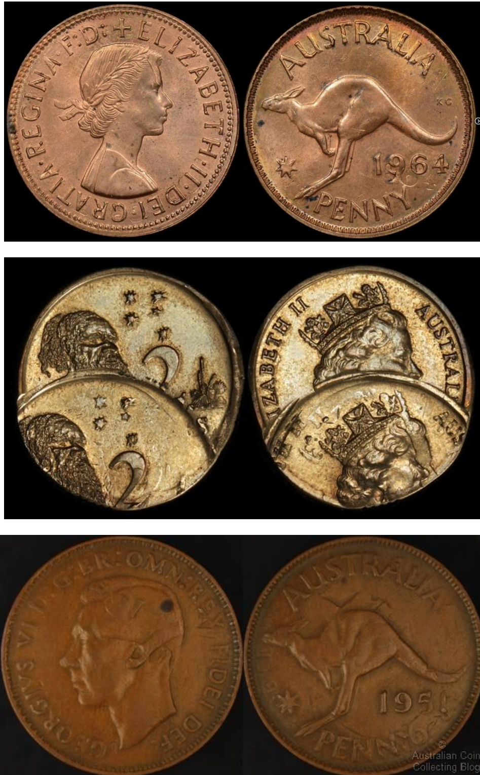
Figure 2 (part). Double strike on centre (top), multiple strike (second from top), flip over double strike (third from top).
