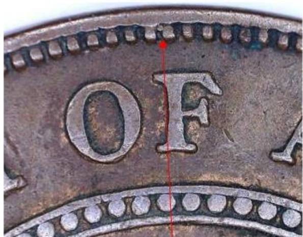
Figure 4. Tiny die chip that appears on the specimen/proof and some of the business strike 1930 pennies. Photograph courtesy of Fred Lever.
