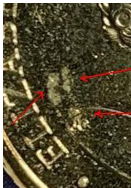
Figure 3. Areas (red arrows) struck through oil or grease on a 2023 $1.
